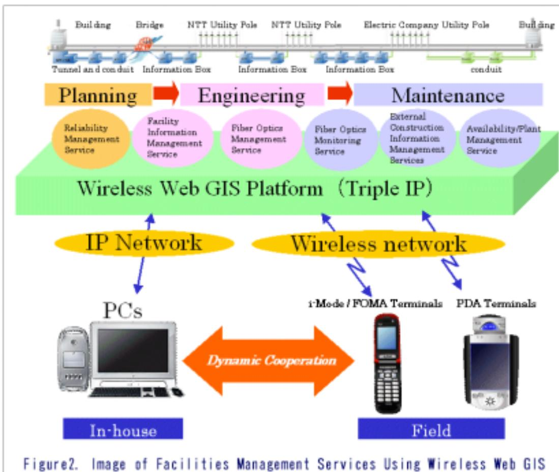
Figure2. Image of Facilities Management Services Using Wireless Web GIS
